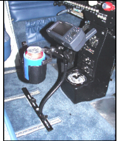
RAM Seat Rail Mounting System holding a Garmin 295 GPS & a RAM Self Leveling Drink Cup Holder.
