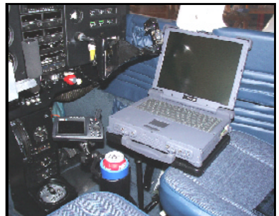
RAM Seat Rail Mounting System holding a Garmin 295 GPS, a RAM Self Leveling Drink Cup Holder & a RAM Lap-Top Computer Tray.
