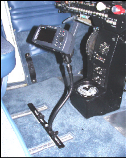
RAM Seat Rail Mounting System holding a Garmin 295 GPS.
